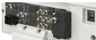
Connector panel with the optional BKM-341HS
