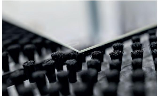
OR-PC®'s have a protective glass pane made of aluminosilicate thin glass as standard. It is highly scratch-resistant and resilient, saves weight and increases display brightness.
