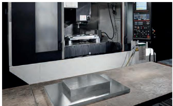
In its own milling shop, OR® produces all-aluminium housings, which have an excellent thermal conductivity and thus, as passively cooled housings, enable a long life of the electronic components.
